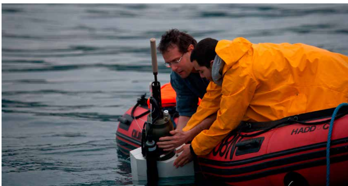
Figure 15: Bio Argo float deployment (© LOV)
