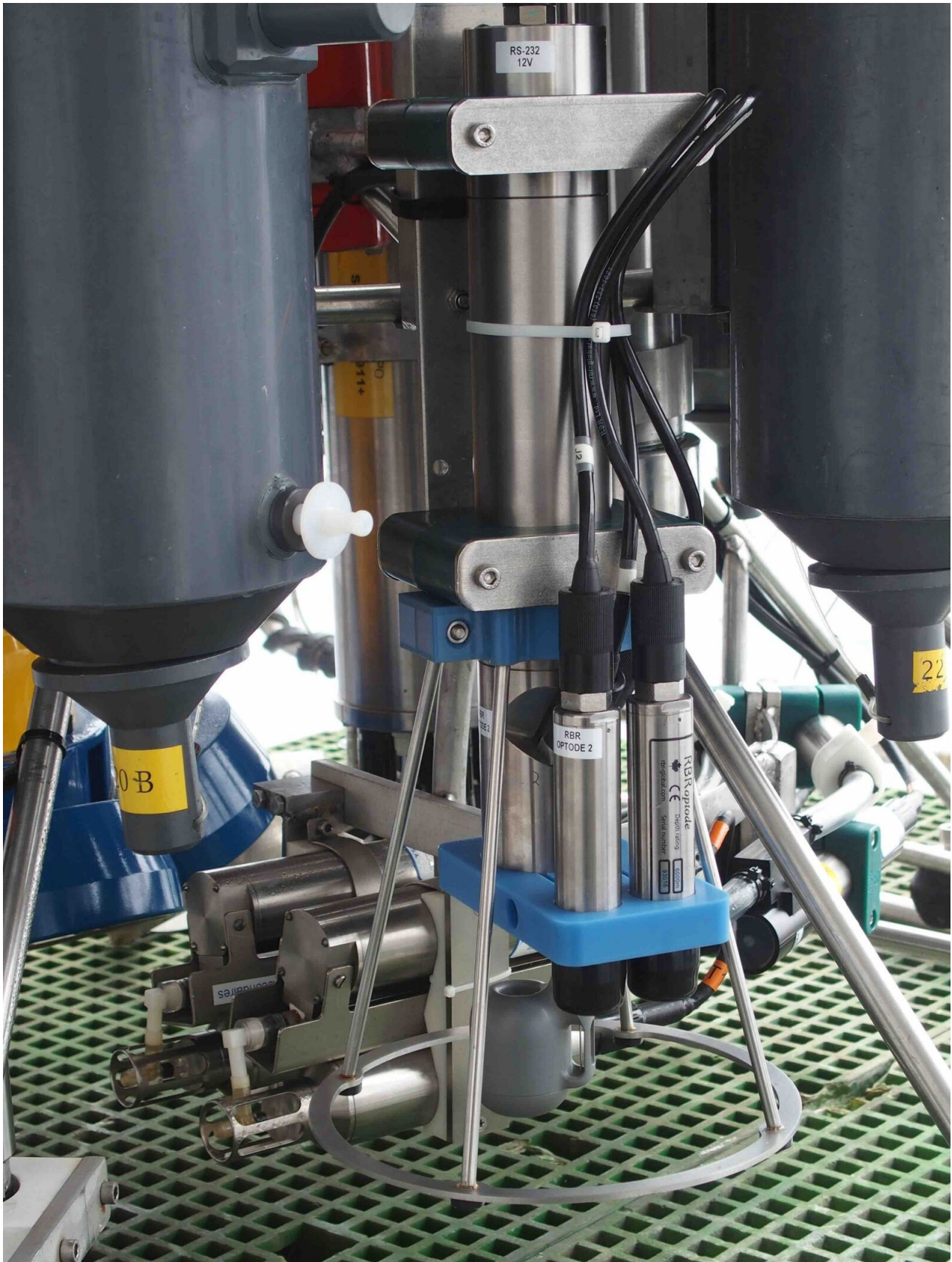
Setting on the LOPS-Ifremer rosette for the test of the deep RBRconcerto CTD (equipped with 2 RBR Optode 2 oxygen sensors). The RBR ctd is mounted near the SBE911.
