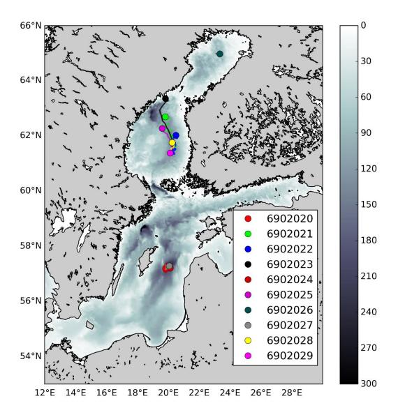
Figure 1, Routes of Argo floats which operated in the Baltic Sea in 2016-2017. Large dots indicate the recovery point or the position of the last profile.
