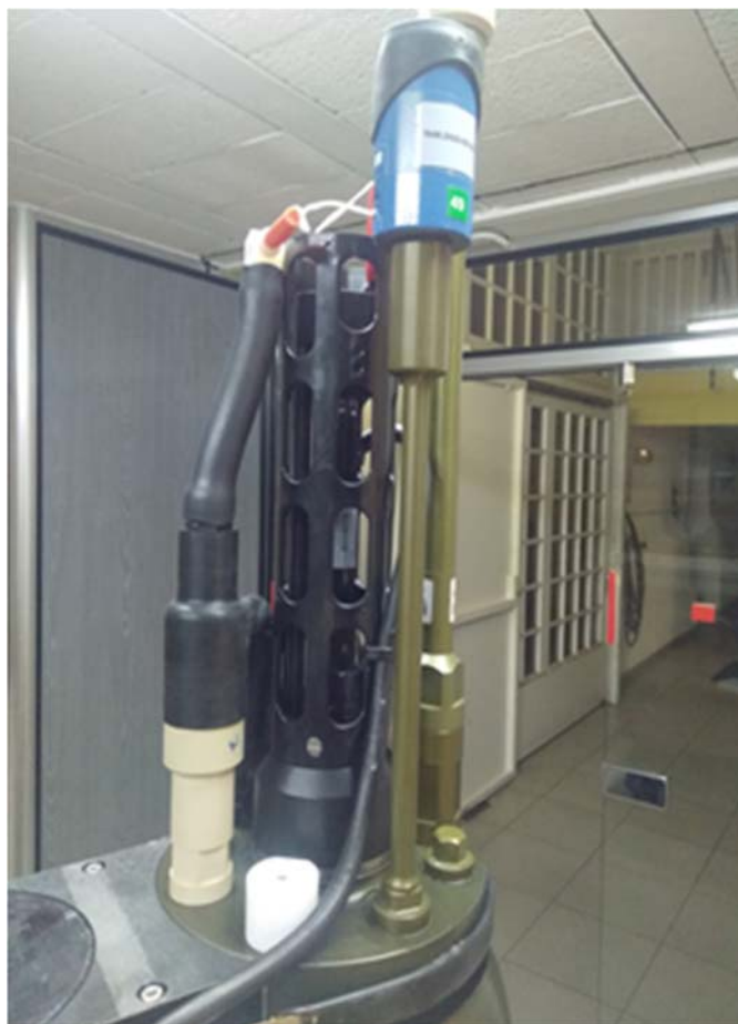
Figure 16. SeaFET pH sensor integrated on a NKE Instrumentations Provor CTS5 profiling float equipped with the OSEAN board.
