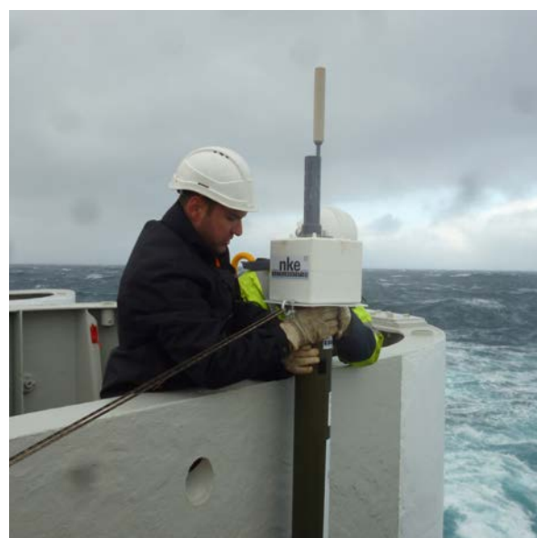
Figure 7: Deployment of an Argo float from cable ship René Descartes in Dec. 2018 (© Orange Marine).
