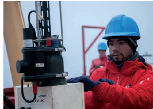
PROVOR-CTS5 float on the icebreaker CCGS Amundsen - GreenEdge Cruise, in Baffin Bay, 2016.
