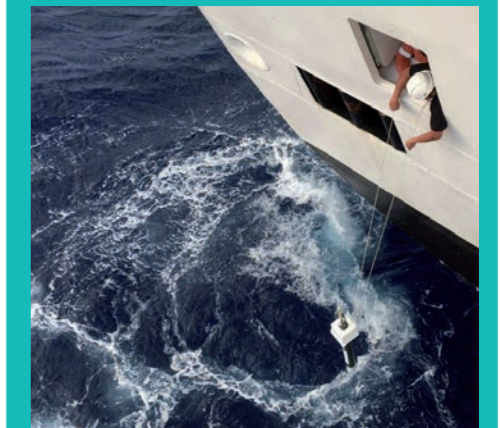
Deployment of an Argo float from cable ship Pierre de Fermat, in July 2018.
