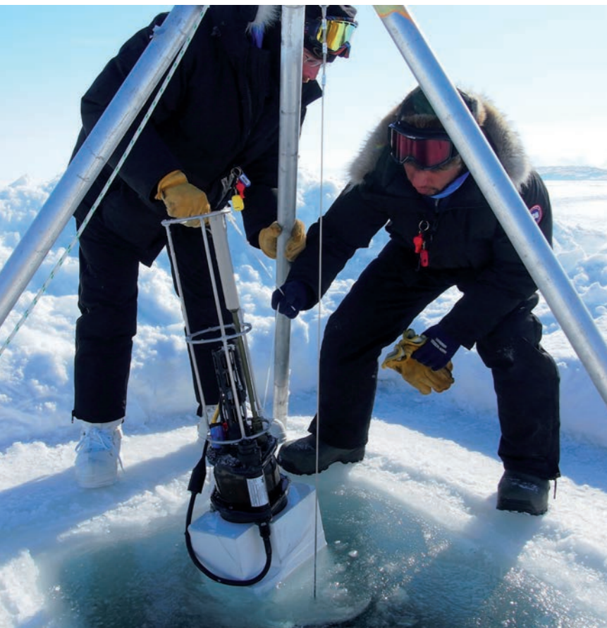
Greenedge ice camp first BGC float with ISA algorithm tested under ice, Qikiqtarjuaq, Nunavut 2015.
