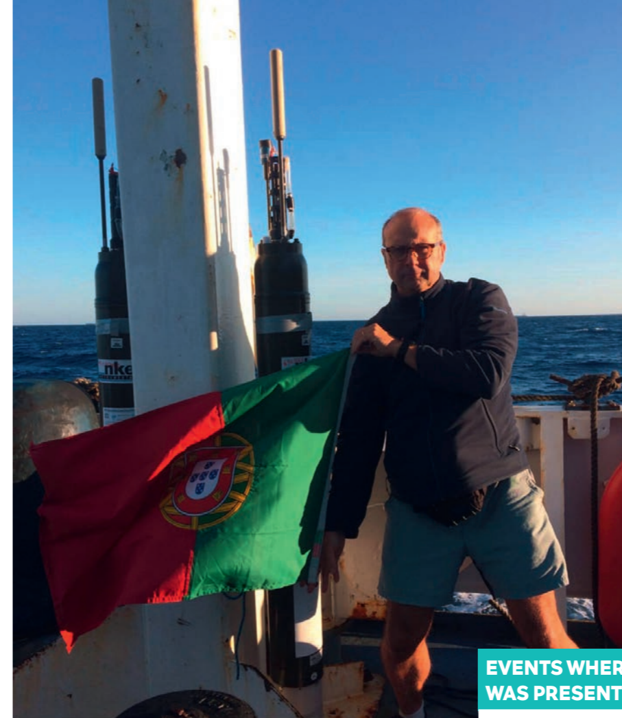
The two Provor floats equipped with oxygen sensors deployed as a collaboration between France and Portugal during the French SHOM PROTEV Gibraltar's campaign.
