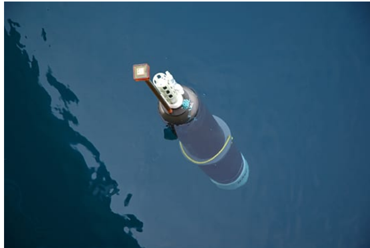
Figure 13: Float with hardened antenna deployed in Arctic from Nevala (2005)
