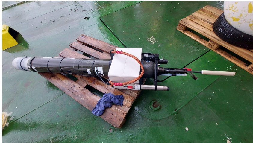
Figure 6: The RAMSES prototype (WMO 6903706) right after recovery onboard Aranda. No signs of biofouling were detectable.
