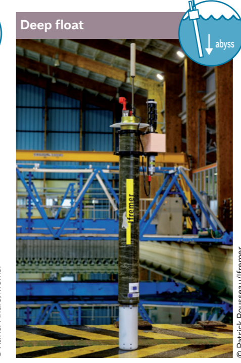
A 2-headed float about to be tested at Ifremer facility to compare the two new sensors (SBE61 on the right, RBR concerto new sensor on the left). This new generation of sensors has been developed in collaboration with Argo international and the manufacturers to provide data accurate down to 6000m.
