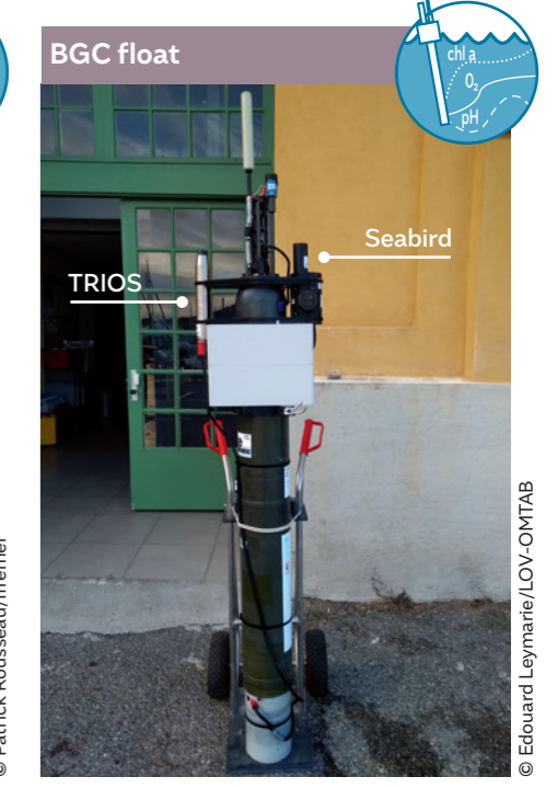
A BGC float was deployed offshore Villefranche, France, to compare two irradiance sensors: the RAMSES hyperspectral sensor from TRIOS and the standard OCR sensor from Seabird. Euro-Argo RISE reinforced the leadership of EU teams in BGC Argo activity.
