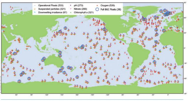
Latest locations of the 533 operational BGC floats in May 2023 and the sensor types they are equipped with.
