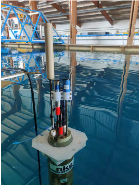
Qualification of the Deep-Arvor profiling float, equipped with both Aanderaa 4330 and Rinko AROD-FT oxygen sensors, for in situ comparison purposes.
