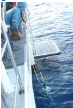
Fig. 1. Arvor with Argos-3 telemetry being deployed in the eastern Alboran Sea on 25 May 2013 from R/V SOCIB.
